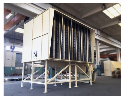
SUPER HEATED WATER BOILER
